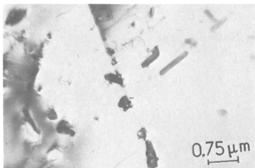
Figure 7 Microstructure of an impure alloy after tempering at 900° C.
